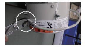
4. Remove the brake release lever pin with a set of pliers.
