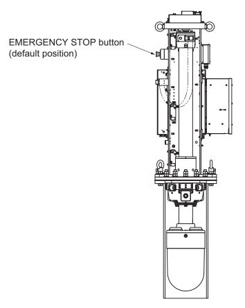
To release the emergency stop condition, first confirm that no one is near the hull unit. Then do the following:
