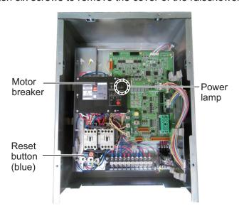
6. Push the RESET button (blue) on the raise/lower control box.
