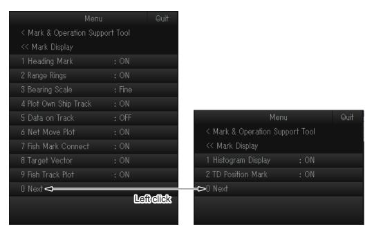
[1 Heading Mark]: The heading mark is a dashed line which indicates the heading in all presentation modes. It extends from own ship position to the outer edge of the display and appears at zero degrees in the head-up mode. It changes the orientation depending on ship's orientation in the north-up and course-up modes.
