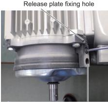
Check that the holes are aligned
