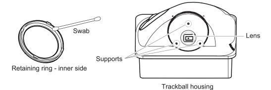
5. Re-set the ball and retaining ring. Be sure the retaining ring is not inserted reversely.
