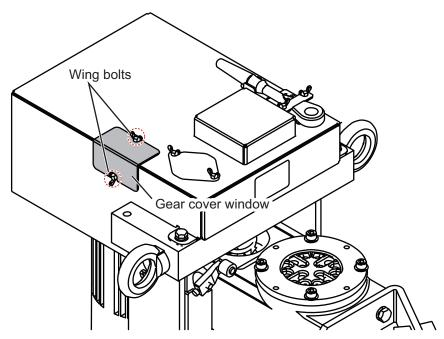
2. While raising and lowering the transducer manually with the ratchet wrench (see section 7.11.2), apply Molytone No.2 grease.
