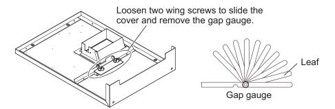
Insert the leaf of the gap gauge horizontally to the place of measurement. Take the measurement. Measure the gap at three places.
